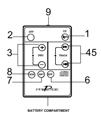
The P-14R Wireless Remote Control (optional) is capable of operating all functions of the wired commander except for the Display Call. Each button on the remote control functions in the same way as the comparable button on the wired commander. For optimal operation of the remote control, always aim it toward the Remote Sensor **bm** on the wired commander.
